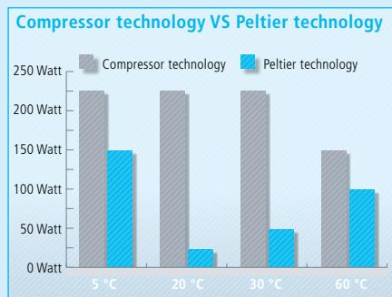
Up to 90 % less energy consumption at 22 °C ambient temperature
