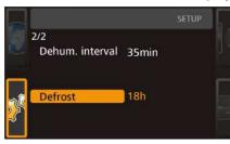
The integrated automatic defrosting system for the cooling unit ensures problem-free operation of the cooled incubator at low temperatures and in permanent operation. The defrosting interval can be set in 6-hour increments, between 6 and 48 hours. The **Off** setting deactivates automatic defrosting.
