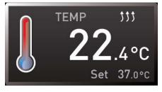
Heating operation is indicated by the 333 symbol. Cooling is indicated by the % symbol.
