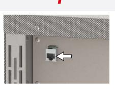
You will find a description of how to transfer programs via Ethernet in the AtmoCONTROL software manual.
