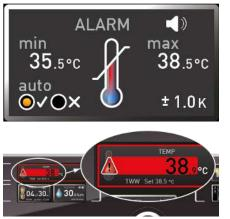
The electronic temperature monitoring measures the monitoring temperature via a separate Pt100 temperature sensor in the chamber. Temperature monitoring settings are made via the **ALARM** display. The settings made apply to all operating modes.
