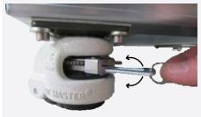
2. To retract and extend the foot, actuate the ratchet lever.
