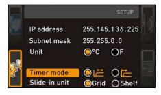
Here, you can choose whether the digital backwards counter with target time setting (see \$\infty 6.5.2 Digital Backwards Counter)\$ should be setpoint-dependent or not – in other words, whether the timer should not start until a tolerance band around the setpoint temperature is reached (a) or if it should start right after activation (a).
