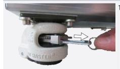
1. To unlock the adjustment mechanism, pull out the ratchet lever on the ring.
