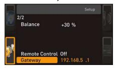
The Gateway setup entry is used to connect two networks with different protocols. The gateway is set the same way as the IP address (see ▶8.3.2 IP Address and Subnet Mask).
