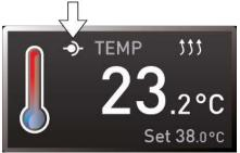
When the appliance is in remote control mode, the  $\mbox{-}$  symbol appears in the temperature display.
