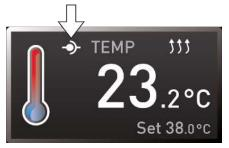
When the appliance is in remote control mode, the  $\mathfrak{P}$  symbol appears in the temperature display. In the settings **Write + Read** and **Write + Alarm**, the appliance cannot be controlled at the ControlCOCKPIT until the remote control has been switched off (**Off** setting) or set to Read Only.
