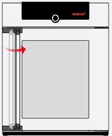
1. To open the door, pull the door handle to the side.
