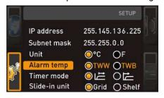
Here, you can choose which temperature protection class in accordance with DIN 12 880:2007-5 should be used (TWW or TWB, description from ▶6.6 Monitoring Function).
