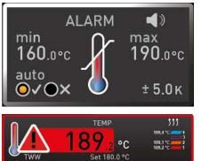
If temperature monitoring has been triggered, this is indicated by the temperature display: the actual temperature is highlighted in red and a warning symbol  $\blacktriangle$  is shown. The type of temperature monitoring that has been triggered is shown beneath the temperature (see > 7 Malfunctions, Warning and Error Messages).
