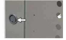
The 8-pin switching output on the rear right post is used to control the vacuum pump of the optional pump module (PM) via the vacuum oven (VO). The switching output is downward-compatible with the 3-pole contact of older pump modules. For this purpose, plug the 3-pole cable into the 8-pole contact.
