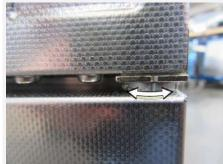
2. Turn the door bearing (eccentric) clockwise or counter-clockwise with a slotted screwdriver as required.
