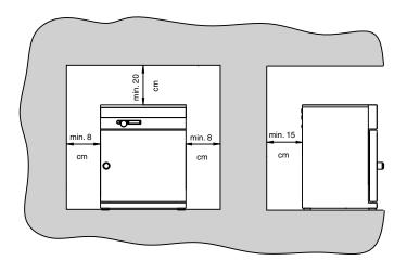
The oven can be placed on the floor or on a bench (working surface).
