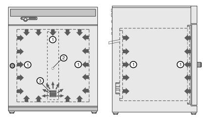
The special feature of the HCP is the particularly uniform conditions inside the chamber. The air is heated by large-area allround heating (1). Humidity is provided by a dry steam generator which produces controlled evaporation of the water. The sterile dry steam is introduced into the chamber above the fan and mixed into the air flow (2). A continuous uniform atmosphere is ensured by the turbulence-free chamber ventilation (3).
