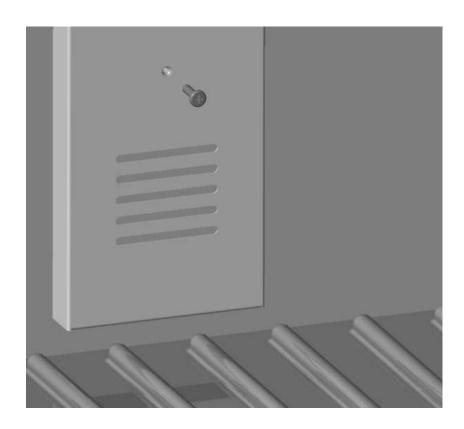
For cleaning of the working chamber the fan cover plate can be taken off the rear wall by removing the screws.
