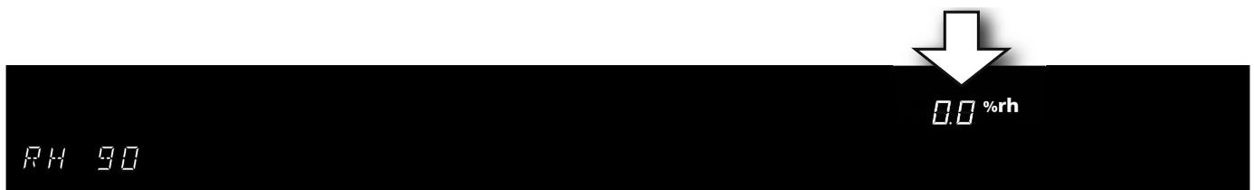
2. With a calibrated reference instrument, an actual humidity of 88 % rh is measured at normal operation, with a set setpoint humidity of 90 % rh.
