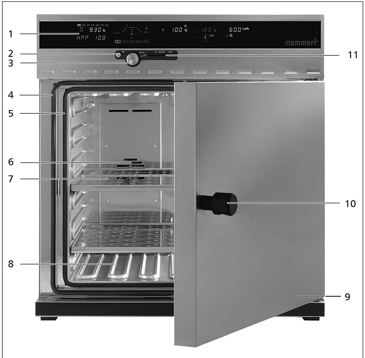
Fig. 2 HPP Constant climate chamber
