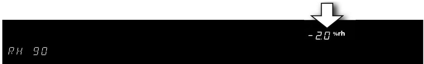
4. The reference instrument should display 90.0 % rh after the calibration procedure.
