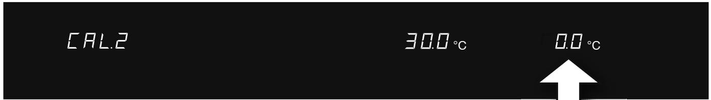
2. With a calibrated reference instrument and at a set setpoint temperature of 30 °C in normal operation, an actual temperature of 29.6 °C is measured.
