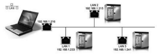
Each device connected to the network must have a unique (IP) address for identification. Each oven is shipped as standard with the IP address 192.168.100.100. The IP address can be altered using the program "XTADMIN" which is located on the "Celsius" CD-ROM.
