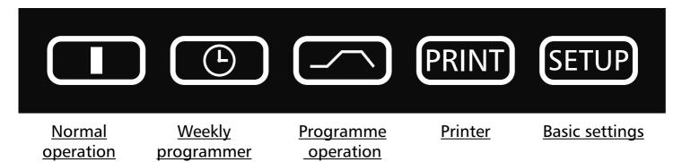
After holding down the SET key (approx. 3 sec), the current operating mode flashes on the display. A different operating mode can be selected with the push/turn control while the SET key is being held down. After the SET key has been released the controller operates in the new operating mode.
