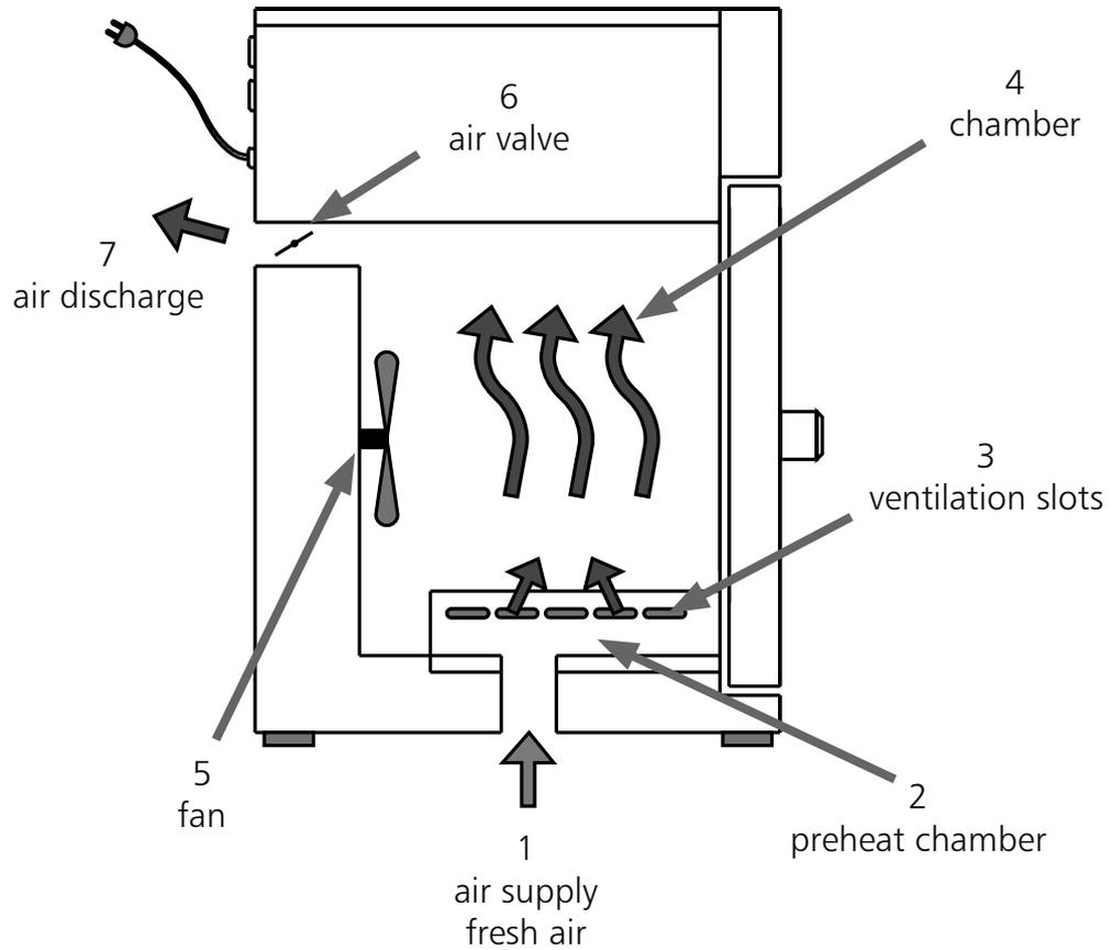
The incoming air (1) is warmed in a preheat chamber (2) in both convection and fan-circulation ovens. The preheated air enters the chamber (4) through ventilation slots (3) in the chamber side wall. The fan (5) on the chamber back wall produces a large air throughput and a more intensive horizontal forced circulation compared with natural convection. The air valve (6) on the back of the oven controls the rate of air intake and discharge (air change) (7).
