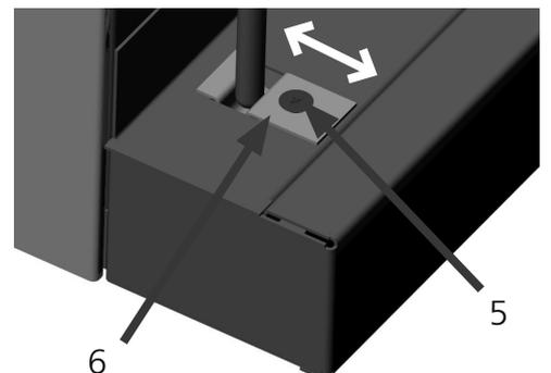
The closing panel (6) can also be adjusted in the direction of the arrow after releasing the screw (5). It is important that the panel is then screwed down firmly.
