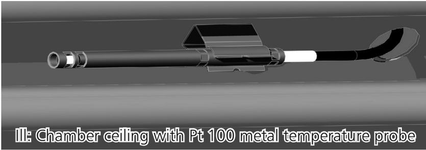
III: Chamber ceiling with Pt 100 metal temperature probe
