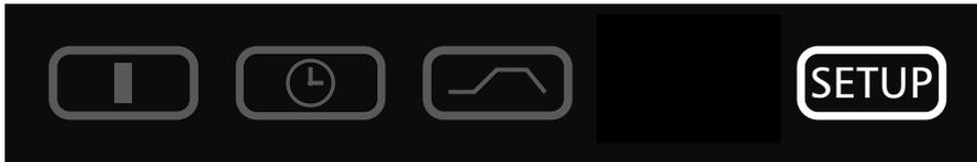
In this operating mode it is possible to make the basic settings for the oven. Clock time, date, day, year and calibration are set here.
