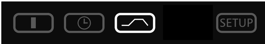
In this operating mode a fixed ramp sequence is programmed. A time period can be input for each ramp segment, or the appropriate ramp segment can be de-activated by setting "----". After the end of the programme the oven switches off the heating and cools down to ambient temperature. In the case of ovens UFE and SFE the fan runs on for 30 minutes.
