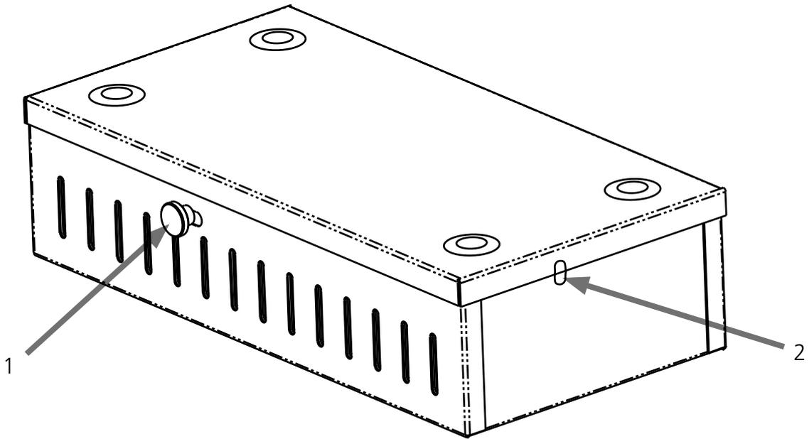
The load to be sterilised is placed into the steriliser cassettes wrapped in aluminium foil or in steriliser foil suitable for hot air (as in the Table in the Section „Guidelines for sterilisation“). The air slots in the cassette must be open for sterilisation.
