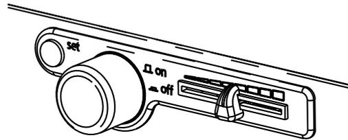
Oven switched on and can be operated using the push/turn control and the SET key.
