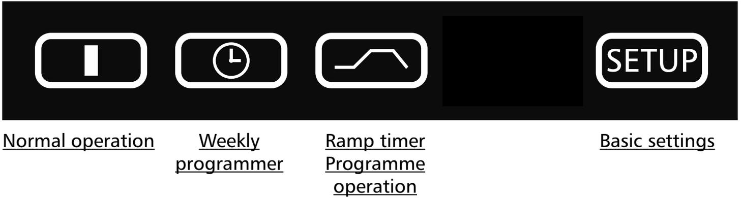
After holding down the SET key (approx. 3 sec), the current operating mode flashes on the display. A different operating mode can be selected with the push/turn control while the SET key is being held down. After the SET key has been released the controller operates in the new operating mode.
