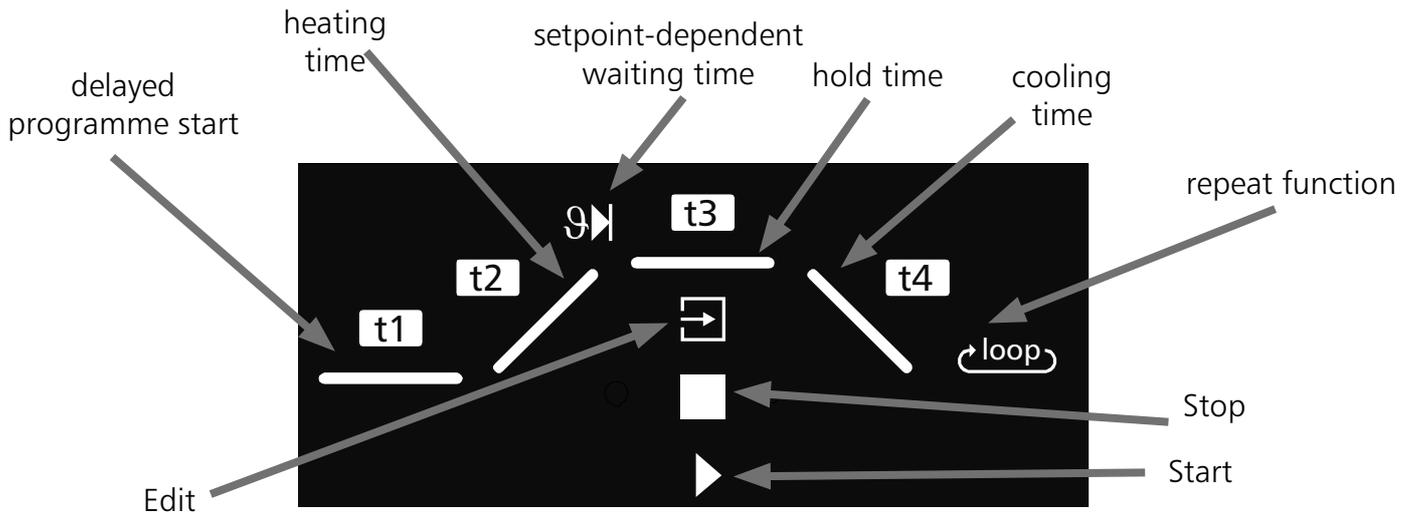
By turning the push/turn control the following parameters can be selected and can be altered as described in the Section „Selecting the parameters“:
