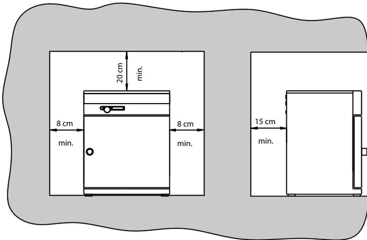
The oven can be placed on the floor or on a bench (working surface). It is important that the oven is set up accurately horizontally; the door may have to be adjusted (see Section: „Maintenance“)
