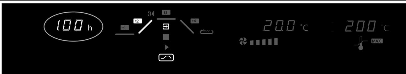
Heating time = heating up to setpoint temperature **t2**
