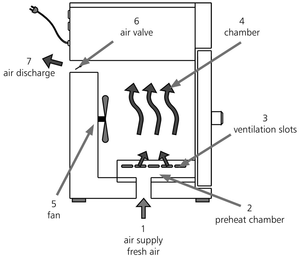
The incoming air (1) is warmed in a preheat chamber (2) in both convection and fan-circulation ovens. The preheated air enters the chamber (4) through ventilation slots (3) in the chamber side wall. The fan (5) on the chamber back wall produces a larger air through put and a more intensive horizontal forced circulation compared with natural convection. The air valve (6) on the back of the oven controls the rate of air intake and discharge (air change) (7).
