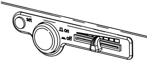
Oven switched off. The push/turn control is pushed in and protected against damage
