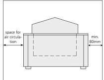
The unit must be placed on a horizontal, non-flammable surface which cannot tilt.
