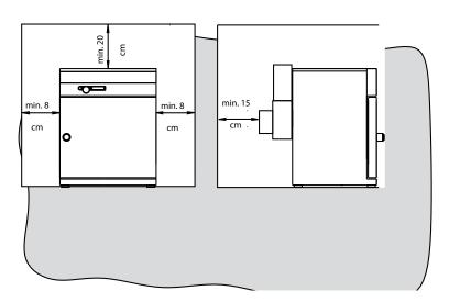
The oven can be placed on the floor or on a bench (working surface). It is important that the oven is set up accurately horizontally; the door may have to be adjusted (see Section: "Maintenance")
