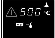
Using the push/turn control select the symbol MIN. Hold down the SET key and set the protection temperature using the push/turn control.
