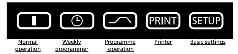
After holding down the SET key (approx. 3 sec), the current operating mode flashes on the display. A different operating mode can be selected with the push/turn control while the SET key is being held down. After the SET key has been released the controller operates in the new operating mode.
