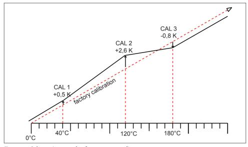
Fig. 28 Schematic example of temperature adjustment
