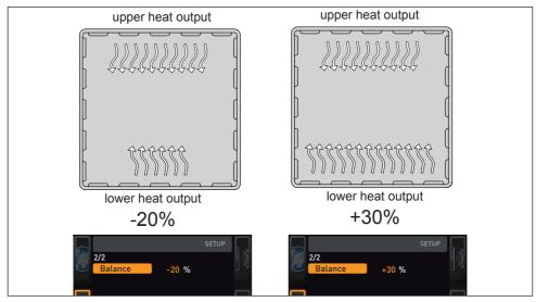
Fig. 27 Heat output distribution (example): The -20 % (left) setting causes the lower heating groups to emit 20 % less heat than the upper ones. The +30 % (right) setting causes the lower heating groups to emit 30 % more heat than the upper ones. The 0 % setting restores the default heat output distribution.
