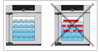
Fig. 16 Correct placement of the chamber load
