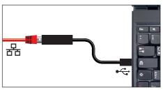
Fig. 8 Converter USB to Ethernet
