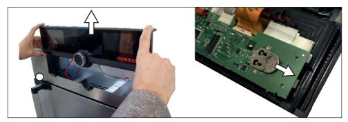
Fig. 30 Removing the lithium battery
