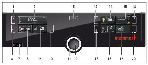
Fig. 18 ControlCOCKPIT for SNxxplus appliances in operating mode (width may differ depending on appliance size)
