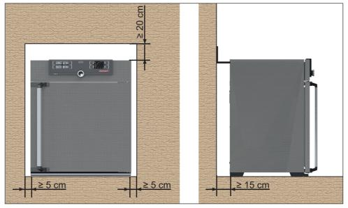
Fig. 9 Minimum clearance from walls and ceiling
