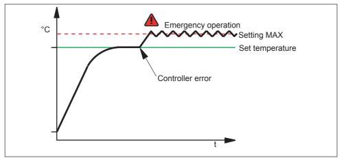
Fig. 20 Schematic diagram of how the TWW temperature monitoring works
