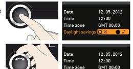
Set daylight savings to off (X) or on (√) with the turn control – in this case on (√). Save the setting by pressing the confirmation key.
