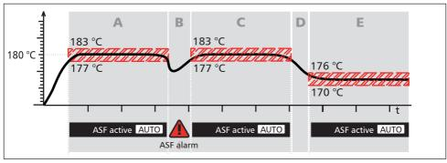
Fig. 22 Schematic diagram of how the ASF temperature monitoring works
