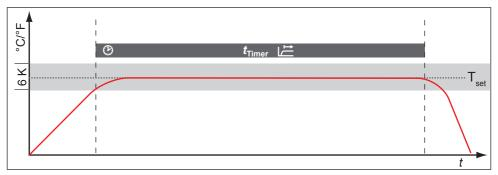
Fig. 26 Timer mode: The timer only starts when the tolerance band of  $\pm 3$  K around the set temperature has been reached
