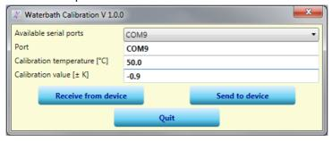
From combobox "Available serial ports" select the port connected to your device. You may then push button "Receive from device" to see the current settings.
