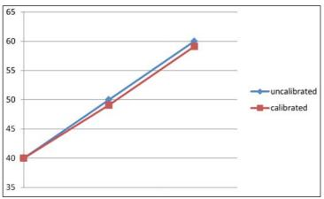
For lower temperatures, the temperatures will be interpolated between the first possible temperature and 50  $^{\circ}$ C. Temperatures higher than 50  $^{\circ}$ C will be constantly decreased by a displacement of 0.9 K.
