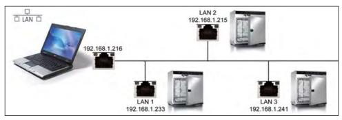
Each oven is delivered by default with the IP address 192.168.100.100. The programme "XTADMIN", which can be found on the USB-Stick, can be used to change the IP address of the oven.
