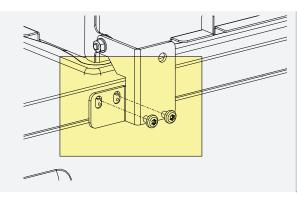
1. Attach brackets for the pipe connection to the back of the water bath.
