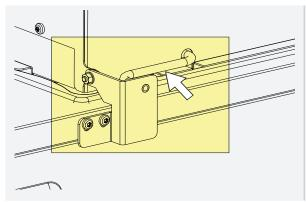
2. Attach the pipe connections to the brackets and hang them in the water bath.
