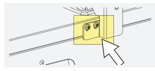
1. Loosen the blind plugs at the fastening points (left + right) for the lid on the water bath.
