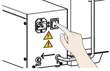
Press main switch on the back of the appliance.
