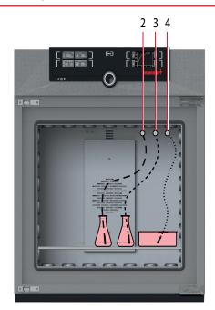
The Pt100 temperature sensor can be flexibly positioned in the interior or in the chamber load to measure temperatures locally (a maximum of 3 additional sensors is possible). The individual temperatures measured are logged in the integrated data logger and shown on the ControlCOCKPIT di play (T2, T3, etc.):
