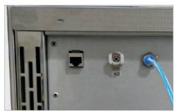
At the back of the device is the compressed-air drying connection.
