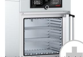
This universal oven made of high-quality hygienic, easy to clean stainless steel leaves nothing to be desired in terms of ventilation technology, control technology, overtemperature protection and perfectly tuned heating technology.
